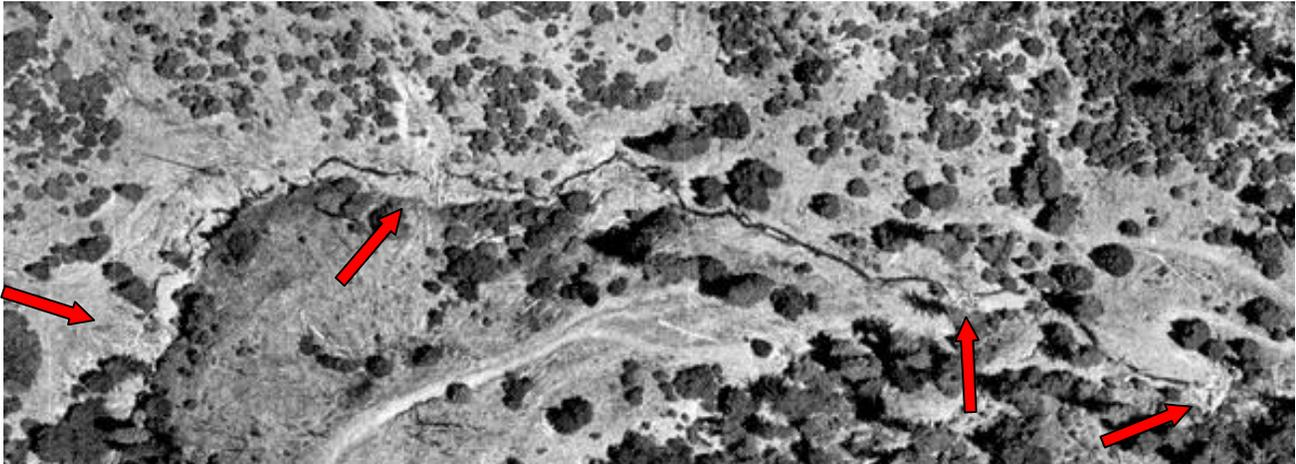
Figure 32 Riparian stream clearance removed coniferous cover in a lower tributary stream to House Creek. These stream crossings (red arrows) also used log chunks pushed into the channel and were topped with dirt fill. The meandering stream channel patterns at the crossings shows the depth of these structures where the stream makes abrupt switchback turns.
