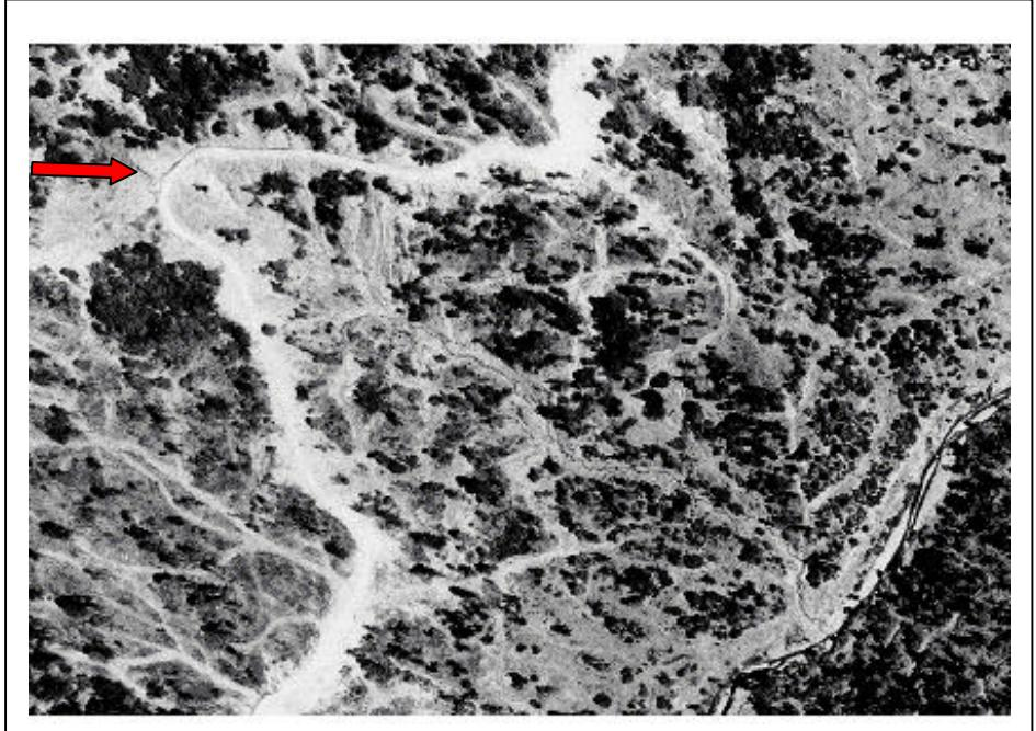
Figure 12: Watercourse diversion down the main road (left) discharged down several skid trails to the lower in stream road. This is a tributary creek to the North Fork Wheatfield, June, 1965.
