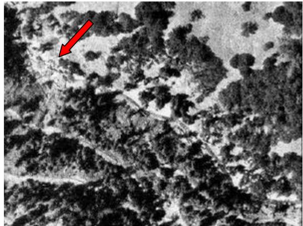
Figure 33: Left: A landing complex was built directly into a stream in a tributary to Marshall Creek, using log chunks and dirt fill. The creek flows under the landing complex at the red arrow. Right: An in stream landing disrupts channel flows along Wolf Creek, tributary to Wheatfield Fork (red arrow).
