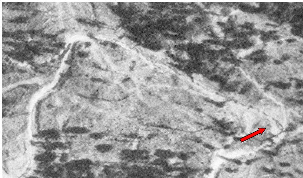
Figure 57: Stream diversion (red arrow) of a tributary stream to the North Fork Wheatfield onto a logging road
