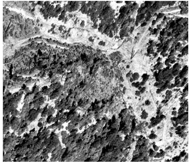
Figure 65: Streamside roads often made several crossings over channel to avoid ungradable obstacles along the streambed in a lower tributary stream to House Creek.
