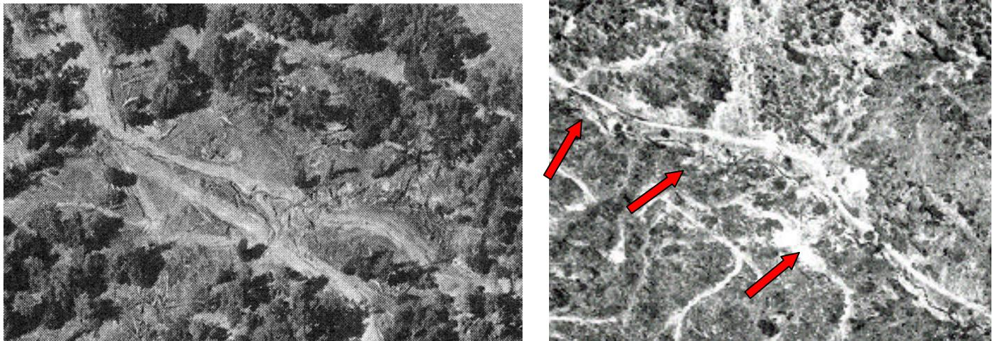
Figure 20: Left: Stream diversion onto a ranch road in the Upper Rockpile PWS, 1965. Rockpile Creek is ~500 feet north. Right: Multiple road debris slides accessing Tobacco Creek.
